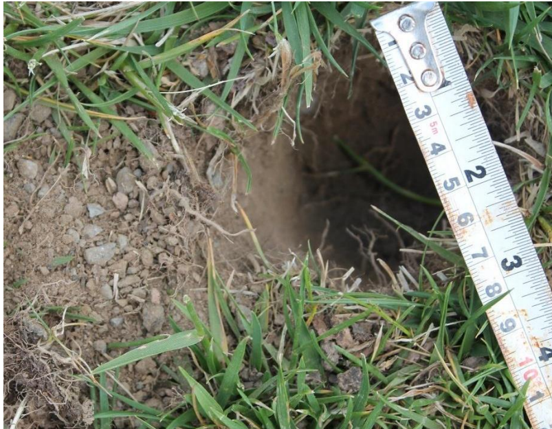
Image 6: Visual inspection of soil profile
